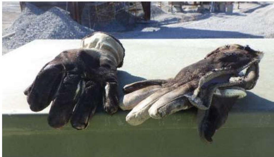
2.21: Burn marks on gloves, evidence of arc flash hazards
