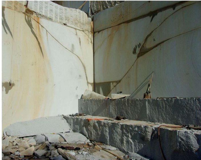
4.7: An accident from loose quarry material occurred because the mine operator did not correct hazardous ground conditions
