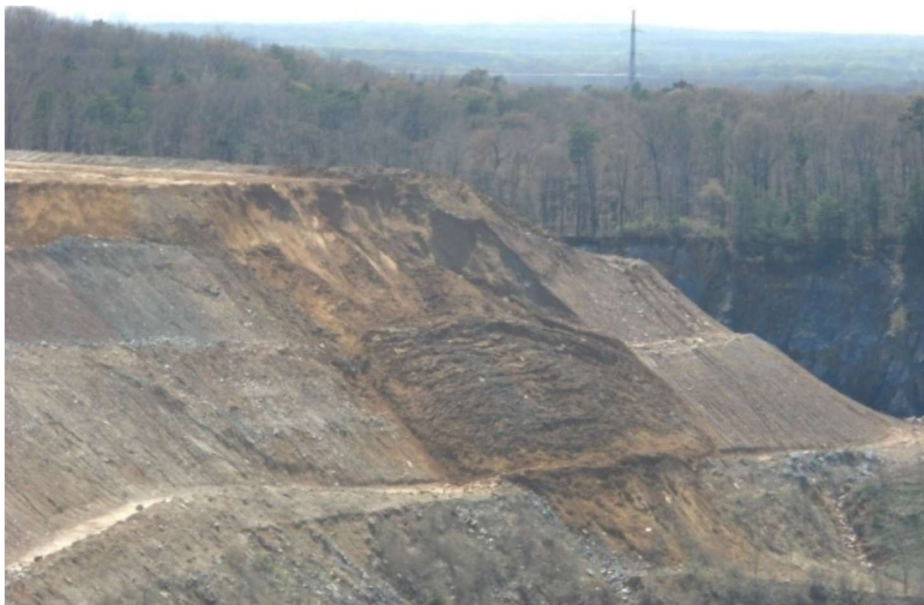
4.1: To avoid dangerous mining landslides (as seen above), use proper tools and methods when scaling any area of a mining worksite.
